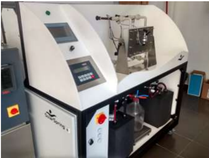
Bench-scale unit for flat sheet membrane distillation testing
