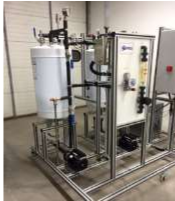
Bench-scale unit for test MD applications in air-gap, permeate-gap and direct contact configurations
